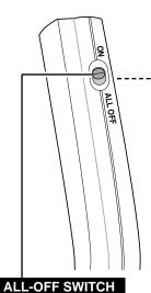
When using Remote Control Unit, turn this switch to "ON." And turn it to "ALL OFF" when it is not used.
